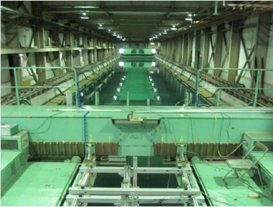
Gambar 4.5 Kolam tarik ( towing tank ) milik Hiroshima University
