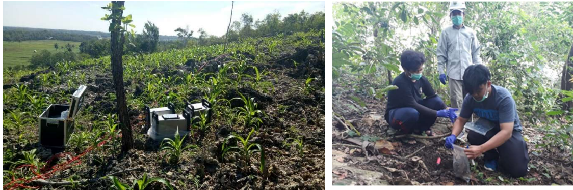
Figure 5. (Left) Resistivity survey equipment. (Right) Soil sampling process.
