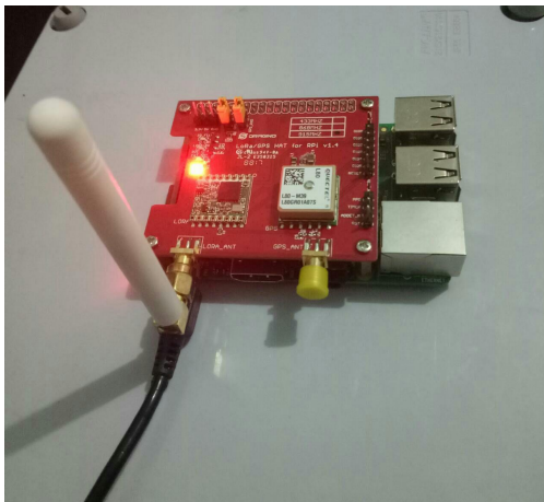
Figure 4. LoRa Gateway / MQTT Broker
