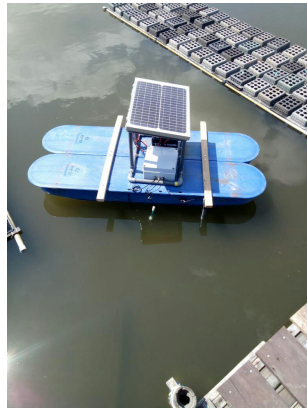
Figure 3. Sensor Node in the pond
