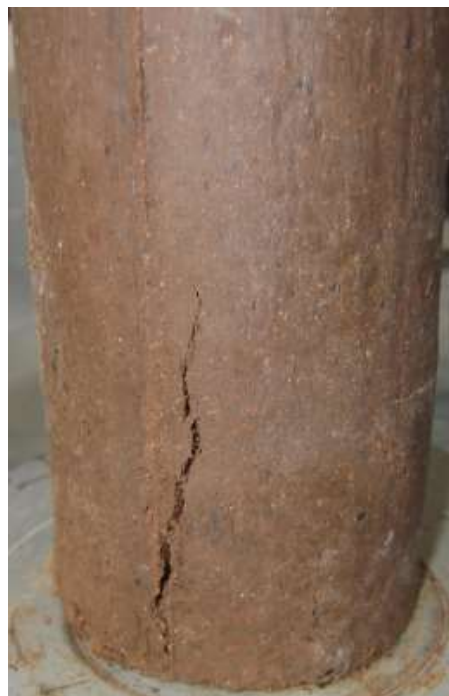
Figure 5. Morphology of Specimens After Compressive Test.
