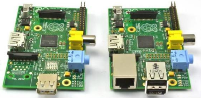
Gambar 5.3 Papan Raspberry Pi Model A (kiri) dan Model B (kanan) ( https://canaltech.com.br/hardware/saiba-tudo-sobre-o-raspberry-pi-3-59065/ )
