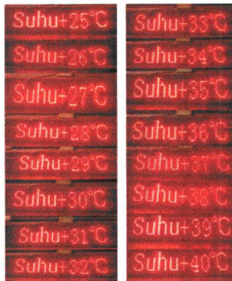
Gambar 5. Tampilan suhu panel LED dot matriks
