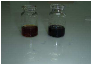
Figure 1. Qualitative test Tannins Using \text{FeCl}_3 Determination of Content of Total Tannins
