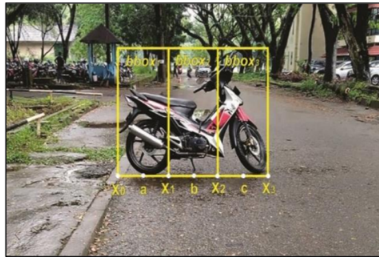
Fig. 10. Bbox division into three parts
