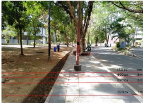
Fig. 8. Initialization of the pixel reference point coordinates in the image
