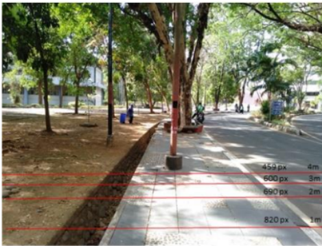
Fig. 8. Initialization of the pixel reference point coordinates in the image
