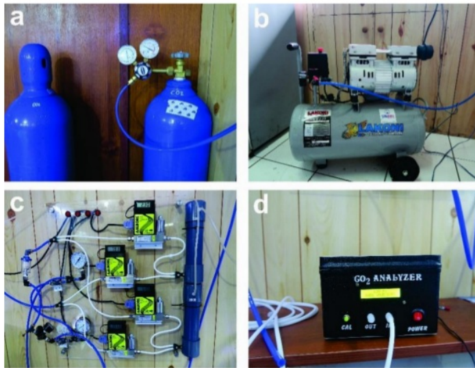
Figure 1. CO 2 system components: (a) CO 2 gas cylinders (b) O 2 compressor (c) Mass flow controller (d) CO 2 meter
