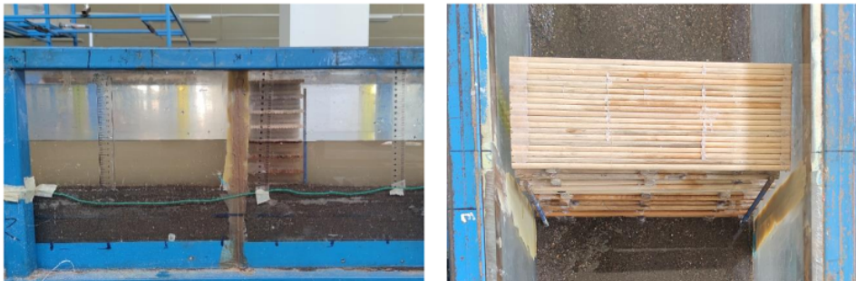
Fig. 4 : In-flume structure HE structure model
