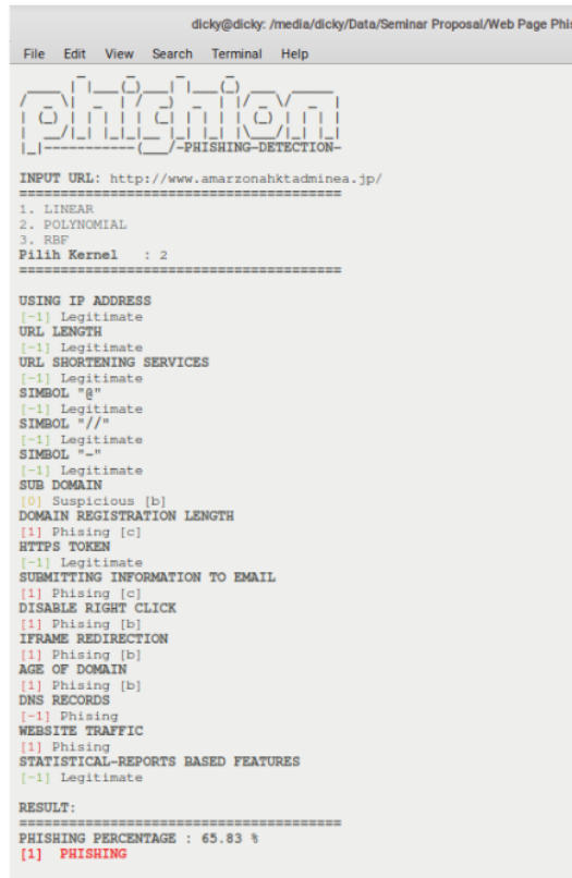
Fig 10. Implementation Results of Phishing Website Detection Program
