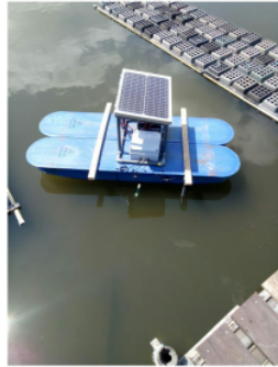
Figure 3. Sensor Node in the pond
