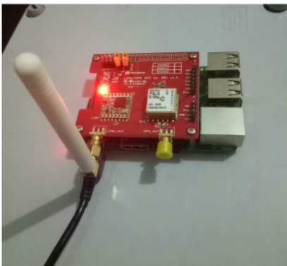
Figure 4. LoRa Gateway / MQTT Broker
