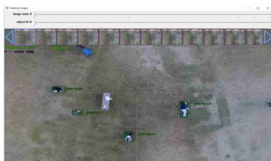
Fig. 4: Labeling images with YOLO_mark
