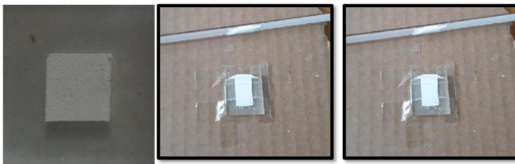
Fig. 2. Paste depositions with the doctor blade method.
